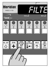
If the controller is programmed for filter lockout, FILTER will appear in the display after the pre-programmed number of cook cycles allowed. The controller will stop operating until the fryer is filtered. After filtering, the display will read FILL. **At this time, the fryer MUST be refilled with oil.** When this step is complete, press ENTER to resume normal operations.
