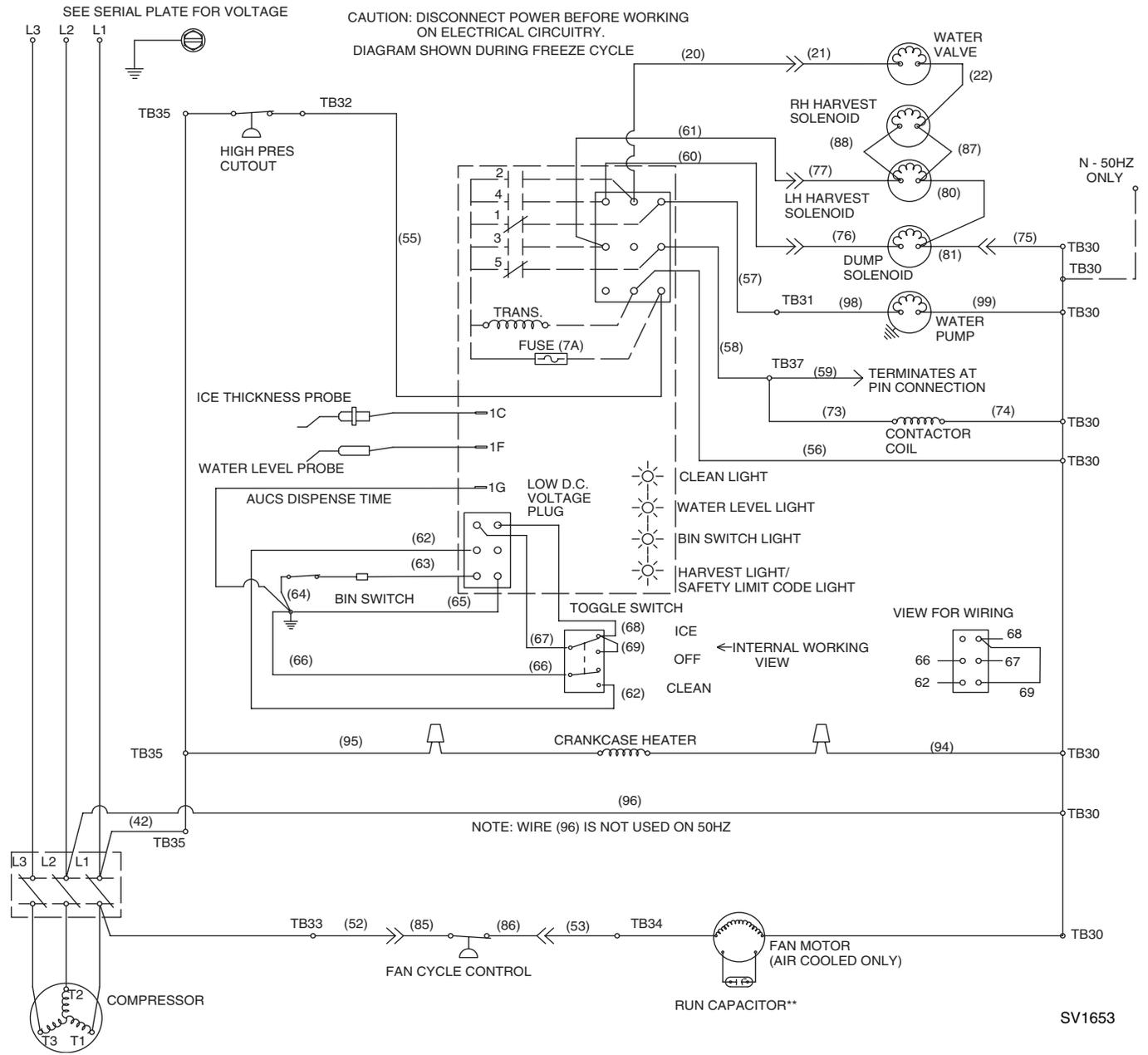
Q1300/Q1600/Q1800 - SELF CONTAINED - 3 PHASE WITHOUT TERMINAL BOARD
