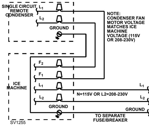
**REMOTE ICE MACHINE WITH SINGLE CIRCUIT MODEL CONDENSER**
