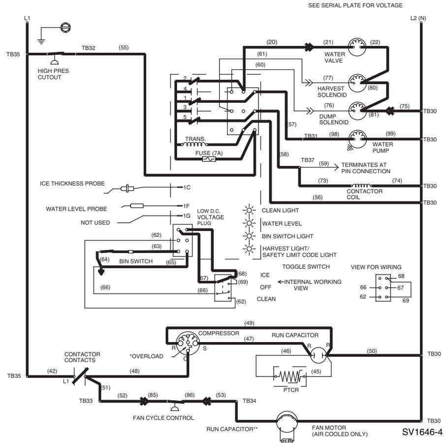
Figure 6-4. Self-Contained — Freeze
