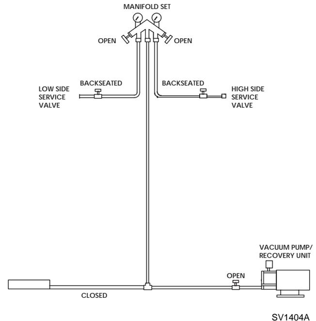
**Figure 7-14. Recovery/Evacuation Connections**
