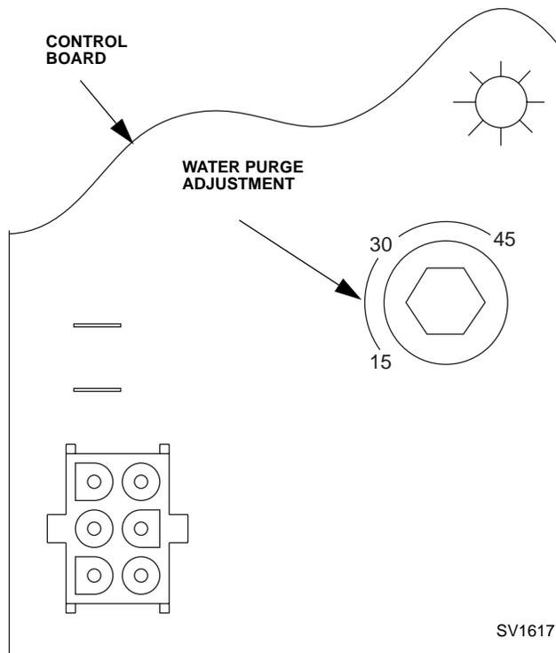
**Figure 3-10. Water Purge Adjustment**
