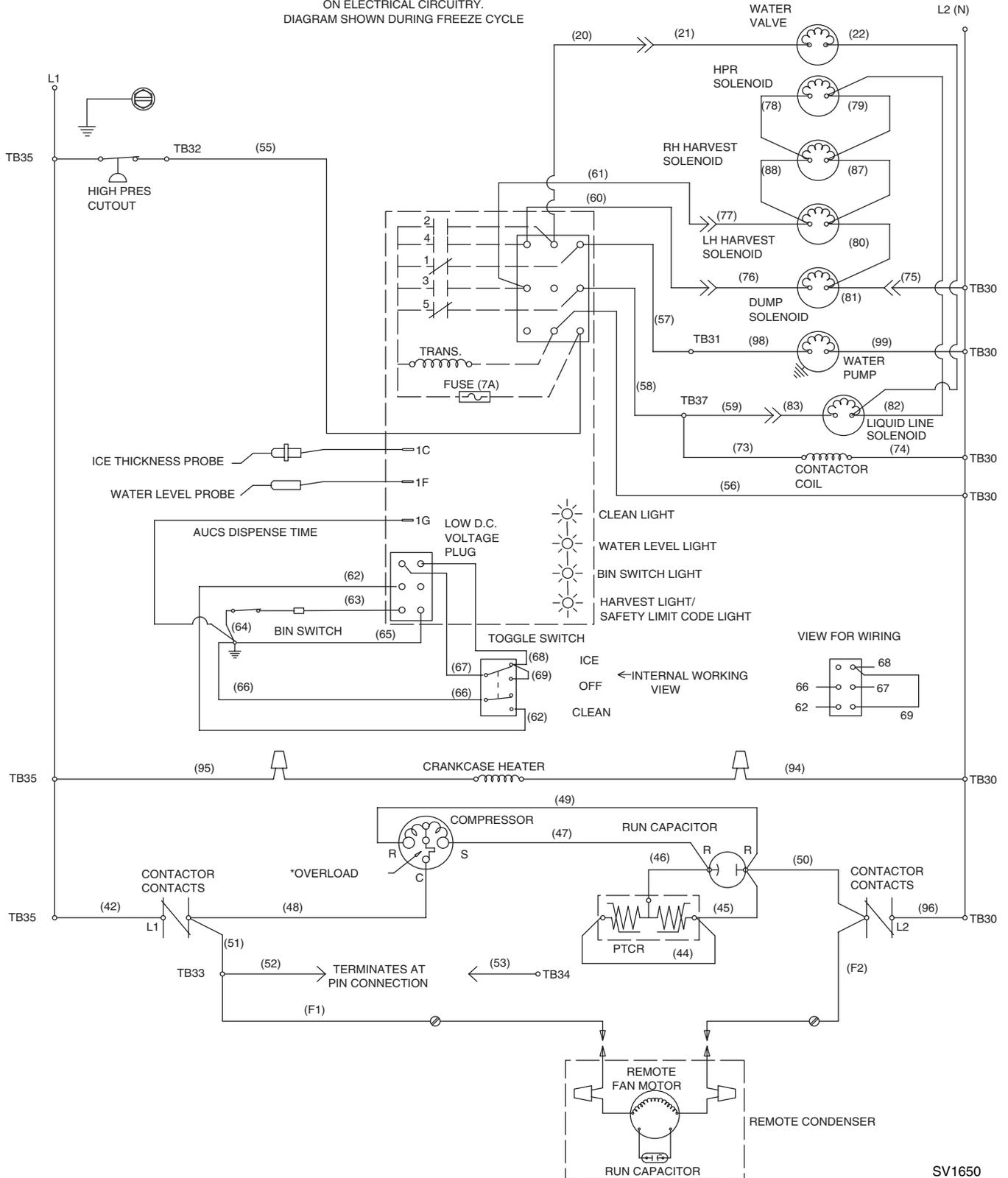
Q1300/Q1600/Q1800 - REMOTE - 1 Phase Without Terminal Board
