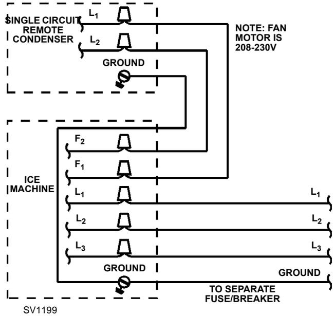
**REMOTE ICE MACHINE WITH SINGLE CIRCUIT MODEL CONDENSER**
