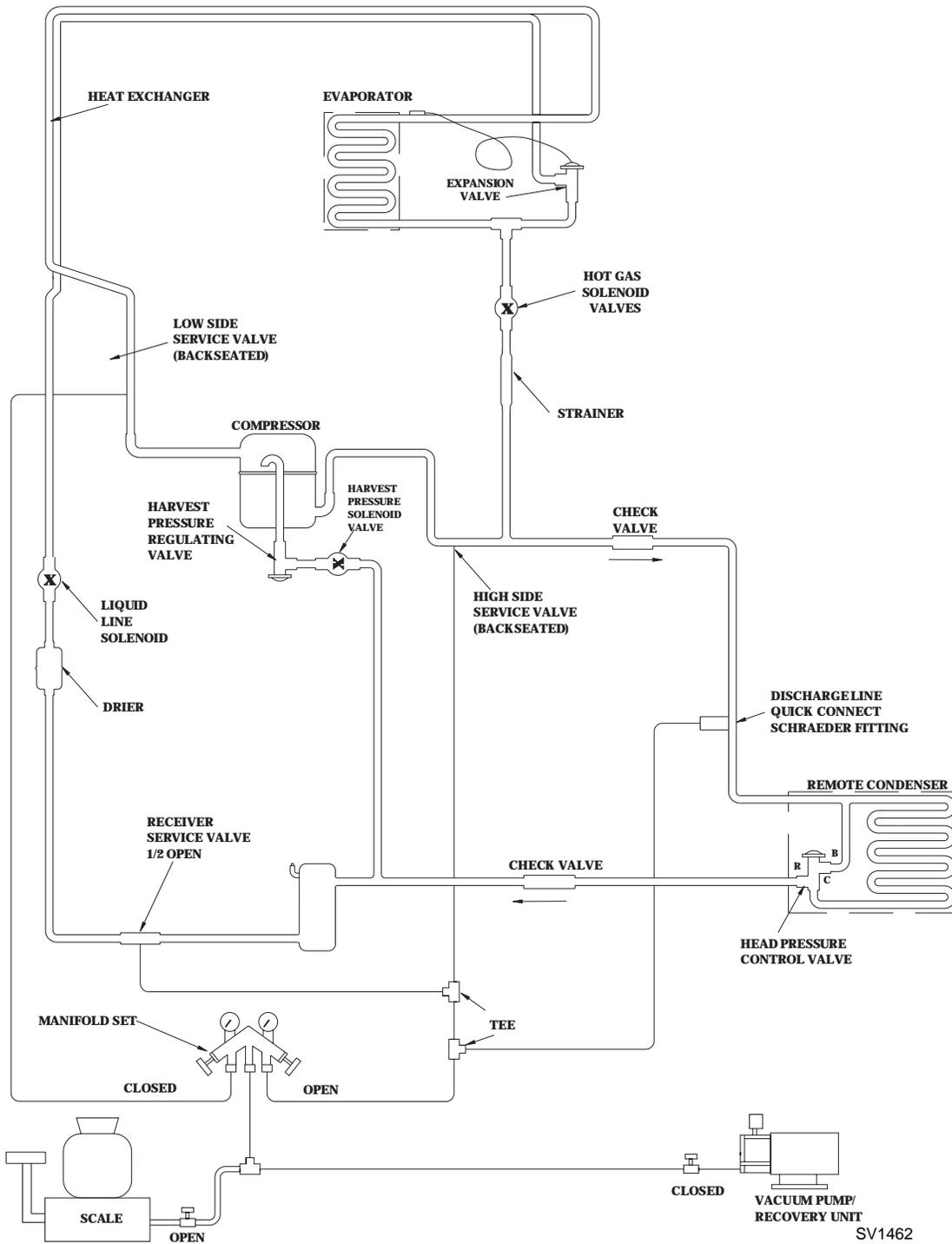
Figure 7-17. Remote Charging Connections
