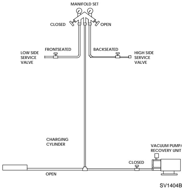
**Figure 7-15. Charging Connections**
