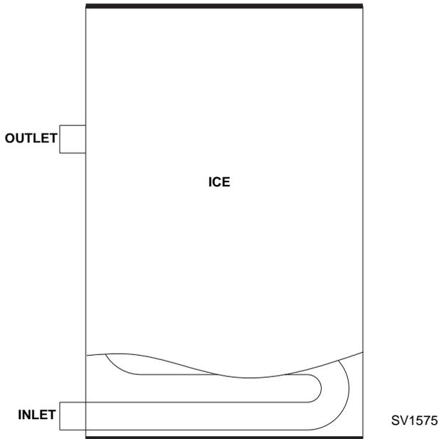
**Figure 7-9. Extremely Thin Ice Formation at Evaporator Inlet**
