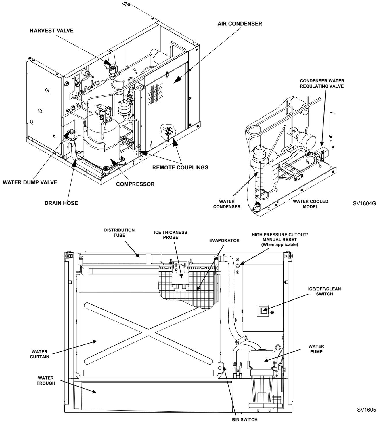
**Figure 3-1. Component Identification (Typical Q450 Shown)**
