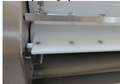
By removing both scrapers, the whole machine is exposed and ready to be cleaned.
