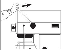
Set the time required by turning the timer to the right. The mixer will stop automatically when the time runs out. Start the mixer by pressing the green start button. The mixer will only start with the timer on and the bowl screen closed.
