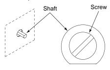
Calibrate the thermostat by holding the shaft in place while turning the screw counterclockwise to increase the temperature, or clockwise to decrease the temperature. Figure 19 -
