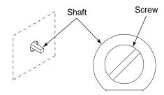
Calibrate the thermostat by holding the shaft in place while turning the screw counterclockwise to increase the temperature, or clockwise to decrease the temperature. Figure 21 -
