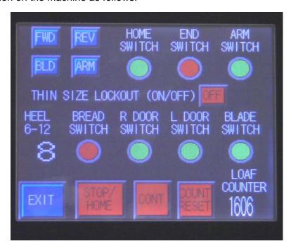
1. FWD and REV buttons move the pusher back and forth. (The covers must be closed to allow movement).
