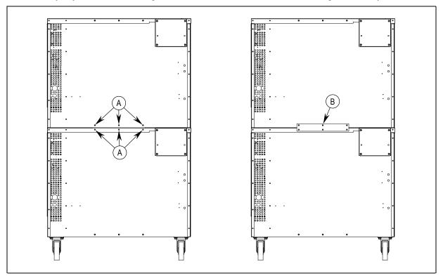
8. Insert two bolts (items "A" in the following diagram) up through the top of the lower oven and screw them into the threaded holes in the bottom of the top oven. Tighten these bolts and the screws that you did not tightened in the previous step.
