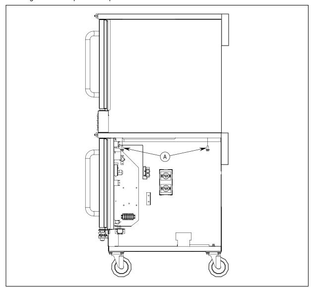
9. Replace the right side insulation, exterior panel, and lower front panel that you removed in steps 3, 4, and 5 of this procedure.
