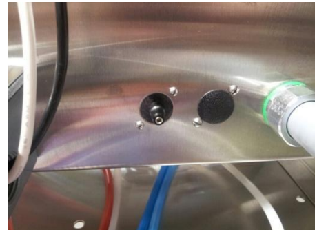
Chemical alarm barb adjusting screw *
