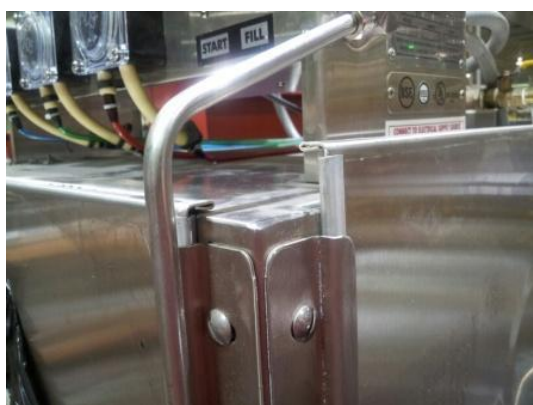
Showing misaligned arms
