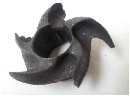
Impeller damaged from high acid solution
