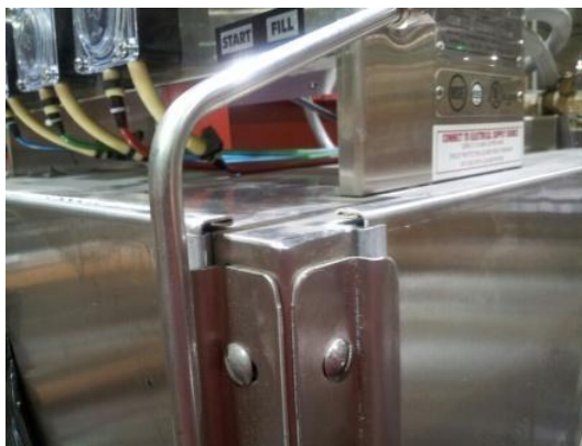
Showing correct arm alignment
