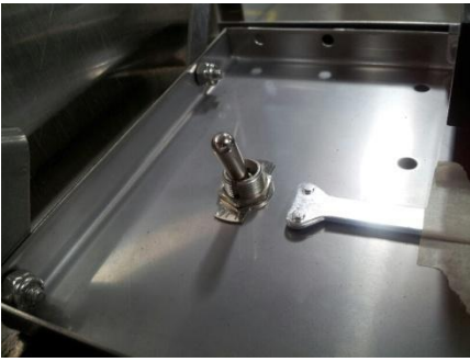
De-lime switch in control box
