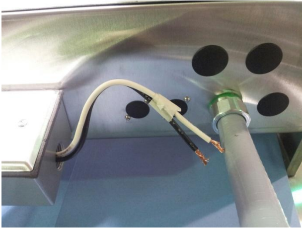
Showing power connection box for 120v wiring
