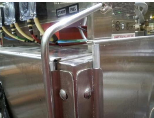
Showing misaligned arms
