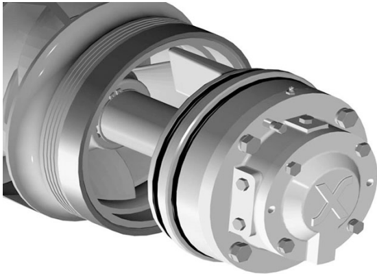
Figure 53: Bearing gland installed on bearing body
