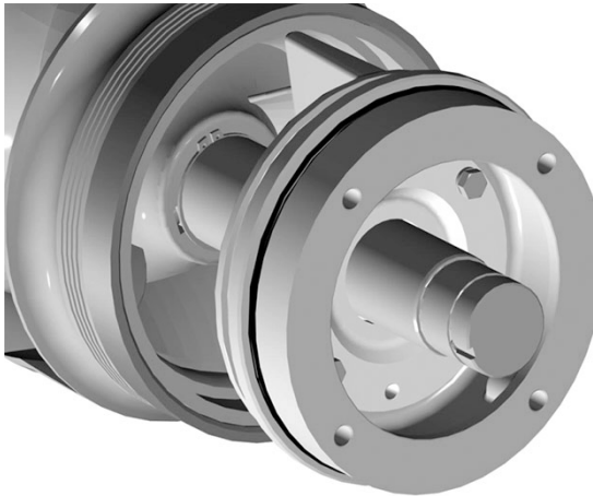
Figure 49: Seal body (stuffing box) with seal gland installed on shaft
