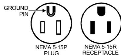
Fig. 3 Plug Configuration
