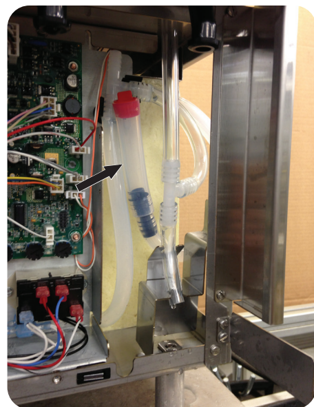
FIG 4 Initial Fill Hose - JDF-4S
