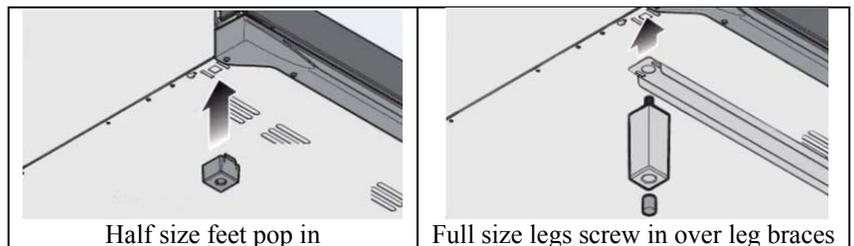
Assemble the feet as shown. (Full size models come with tall legs that screw into place; all other models come with shorter feet that pop into place.)
