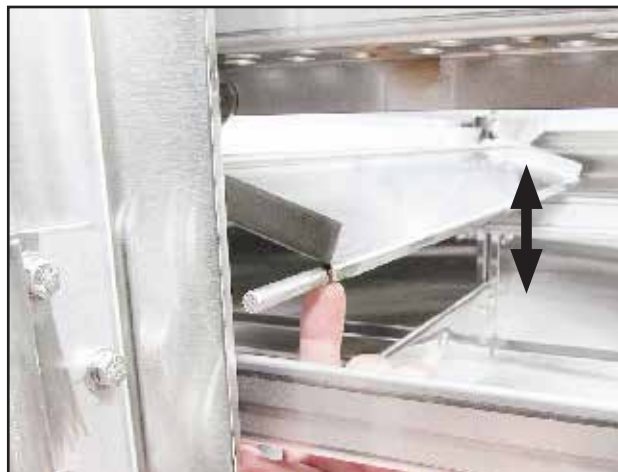
Fig. 9 - Baffles should move freely.
