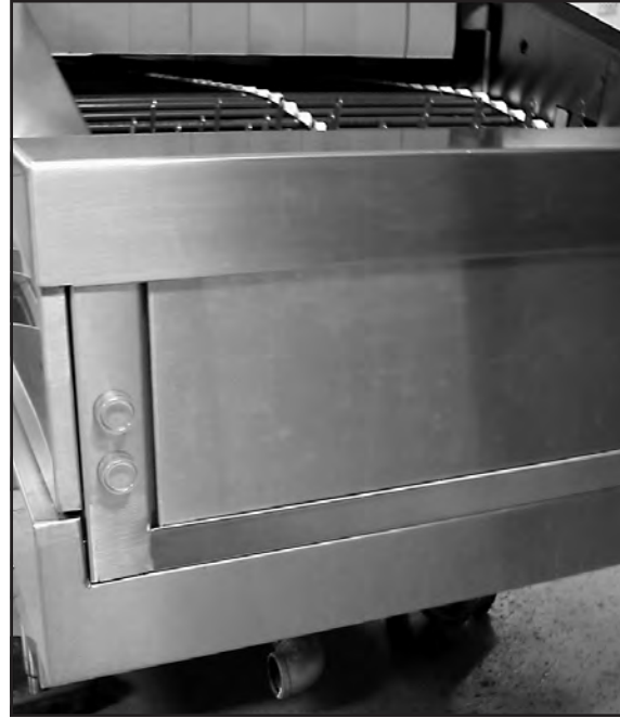
Load-end Start-Stop Station
