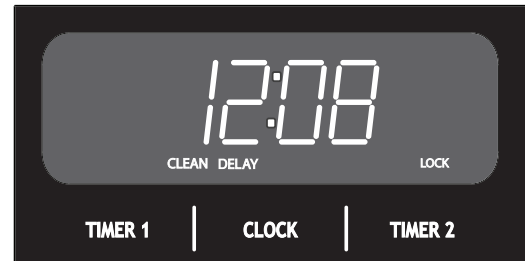
Display When Self Clean Delay is ON
