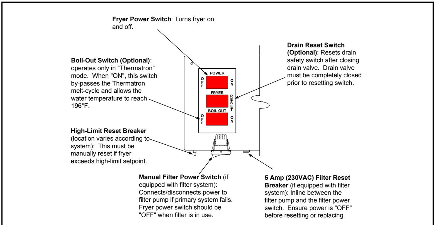
**FRYER POWER SWITCH** – This switch turns the fryer on and off. When the power switch is in the "ON" position, the indicator light will be lit when calling for heat.
