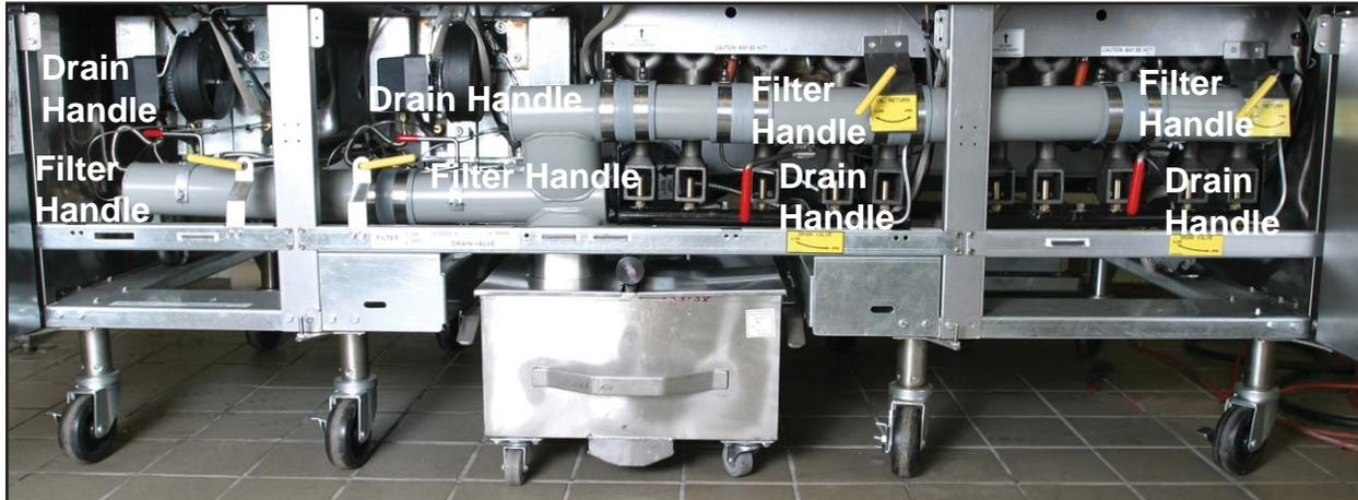
Above is an annotated view of the handles for the filter and drain operation unique to this unit. A quick reference for filtration of the unit is provided to the right and below.
