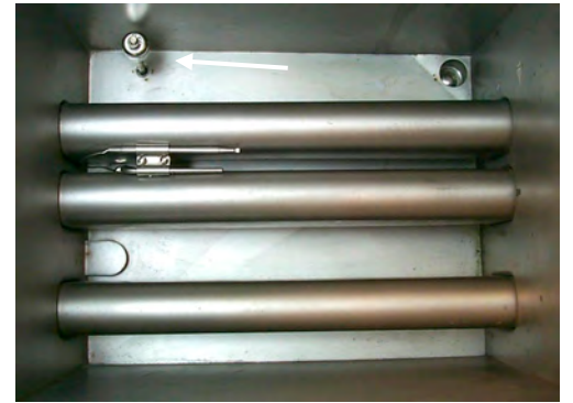
Cook vessel and lower float switch (arrow).
