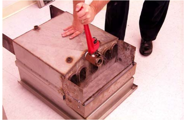
Removing drain valve from frypot.
