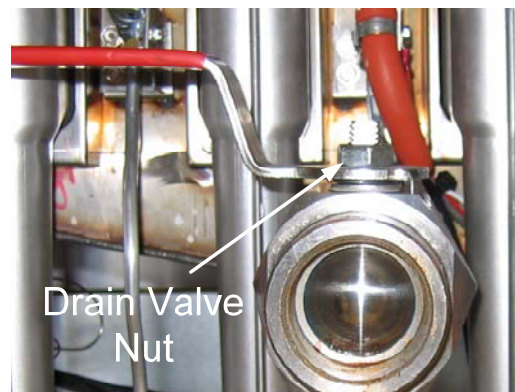
Remove the drain valve nut and attached hardware.
