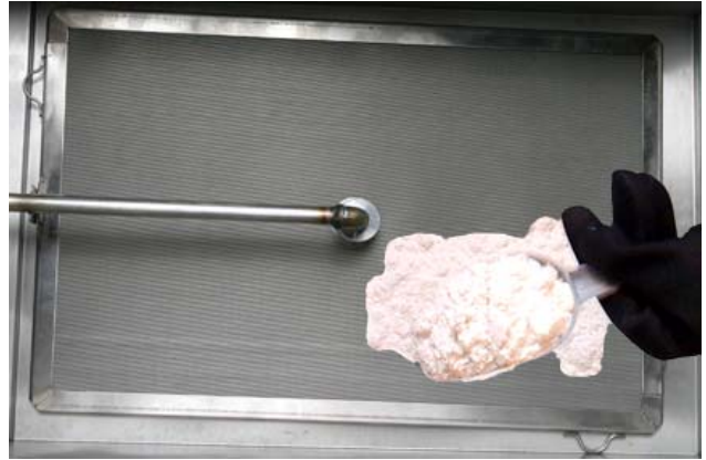
Applying filter powder to filter-leaf.
