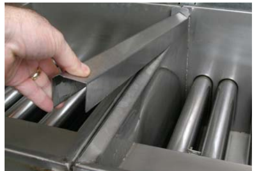
Removing the joiner strip.
