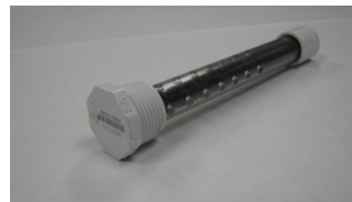
FIGURE 27-2 ODOR CONTROL MEDIA MONITORING TUBE
