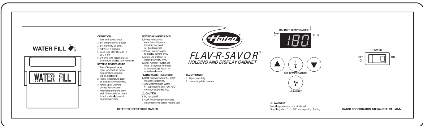
FSD/FSDT Control Panel
