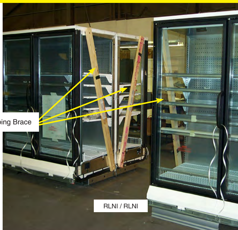
Figure 3. Remove Shipping Braces
