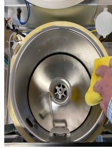
Clean Inside of Hopper
