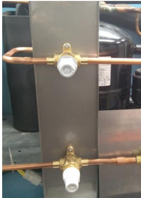
Picture 6: Cut-off valves inside the ice machine
