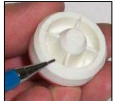
Examining the plunger seating surface
