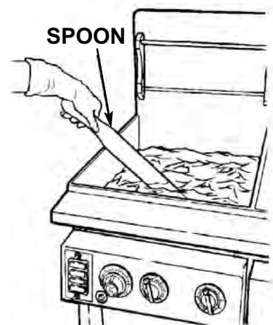
FIGURE 5. STIR WITH SPOON PROVIDED TO REMOVE WATER
