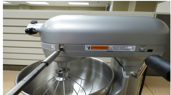
Fig. 38 Mount Upper Housing
