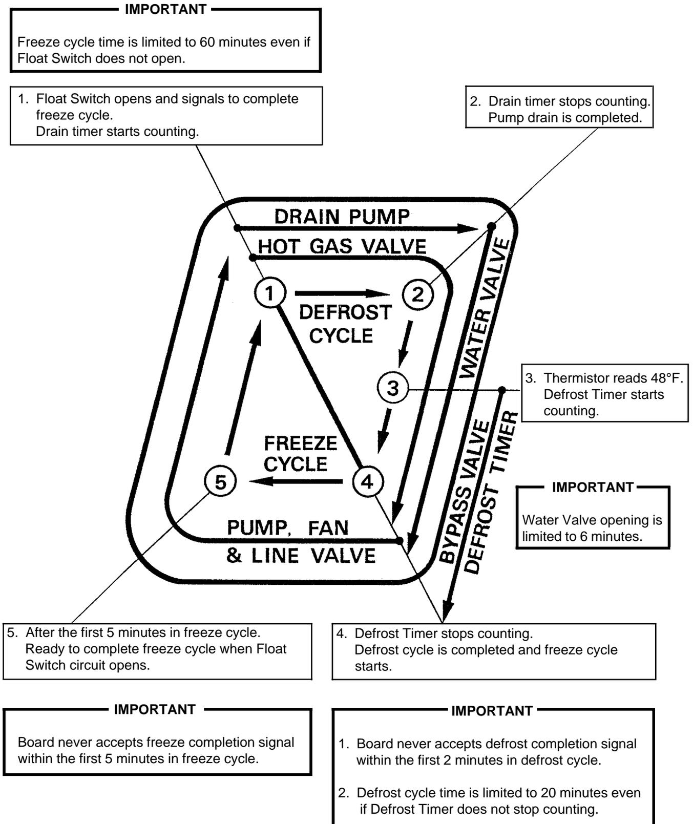
**2nd Cycle and after with no pump drain [KM-1300MRF]**
