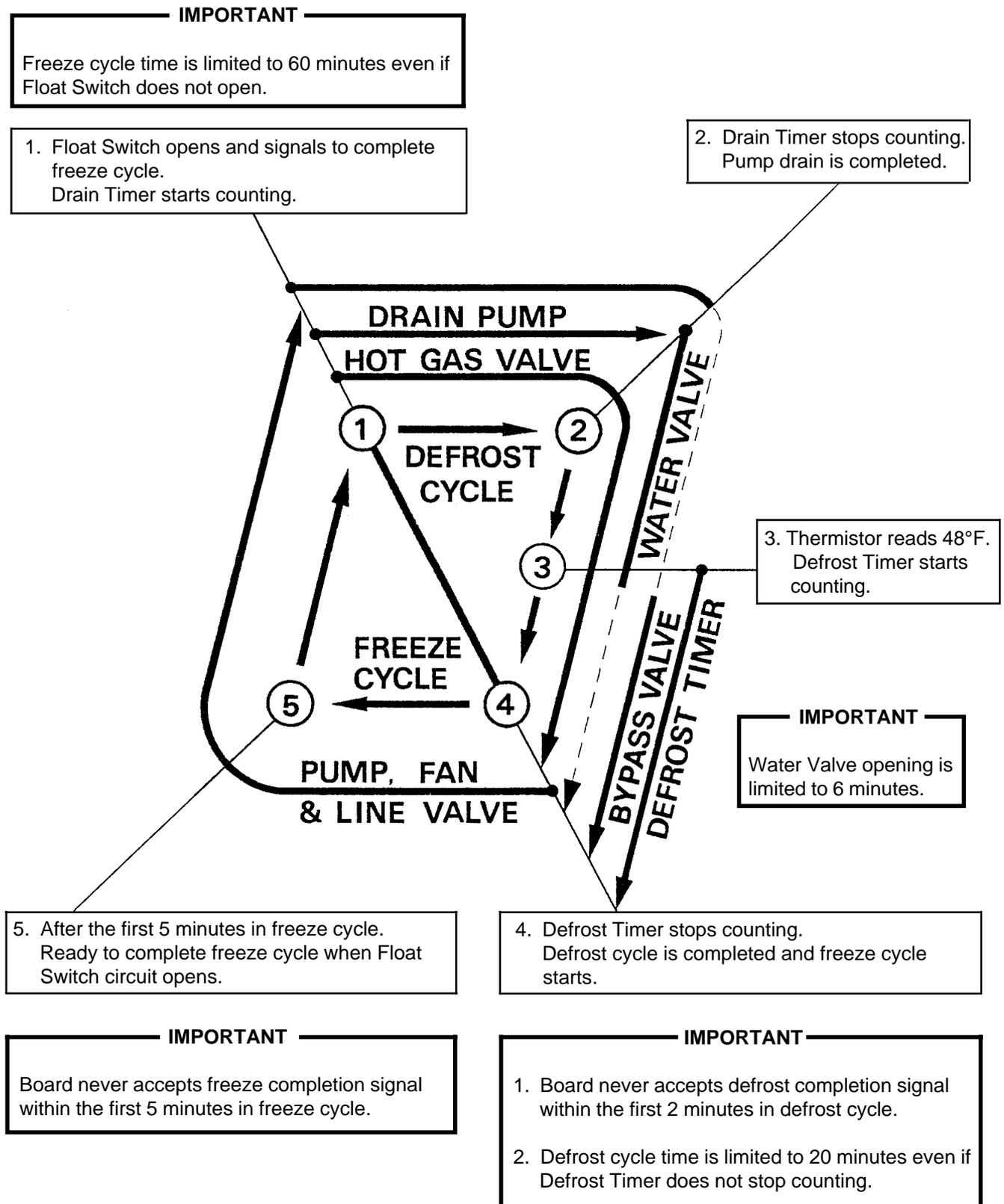
**2nd Cycle and after with no pump drain [KM-1300MAF]**
