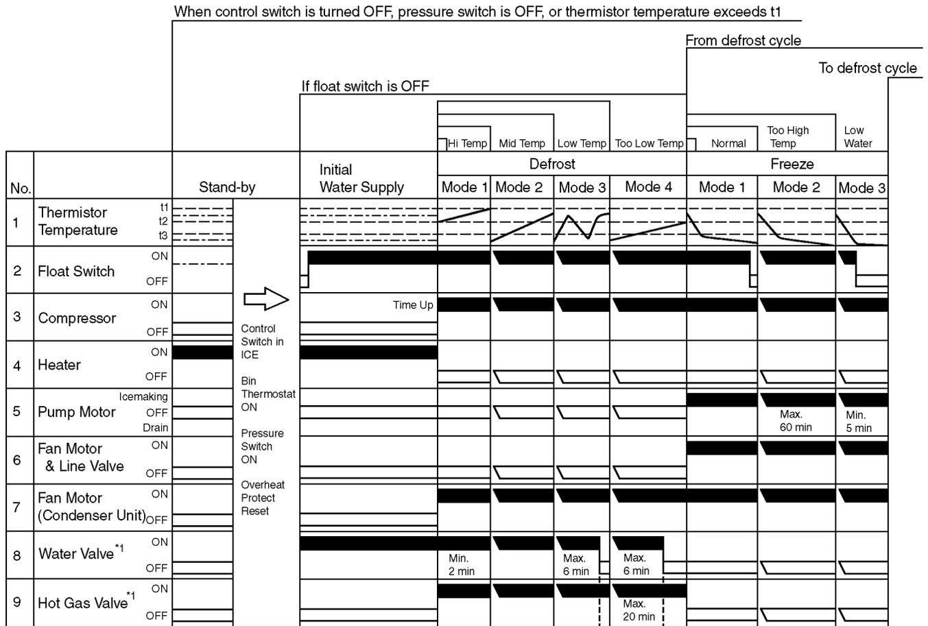
\*1 The icemaker does not complete a defrost cycle in the first 2 or 3 minutes. See "II. 2. [d] Controls and Adjustments."
