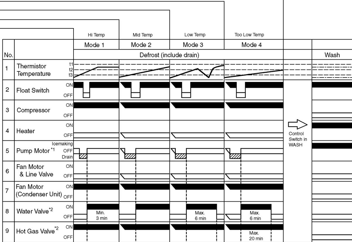
\*1 The pump motor waits for 2 seconds before starting a drain cycle. See "II. 2. [d] Controls and Adjustments."
