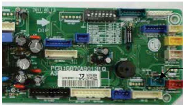
CN-REMO: Remote controller connection
