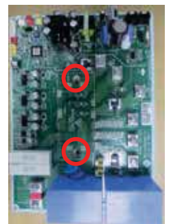
Figure 71: Removing the PCB.
