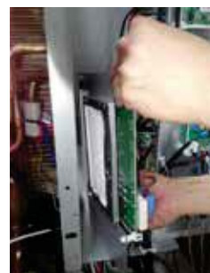
Figure 70: Removing the Inverter PCB.
