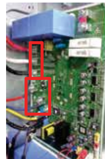
Figure 70: Removing the Inverter PCB.
