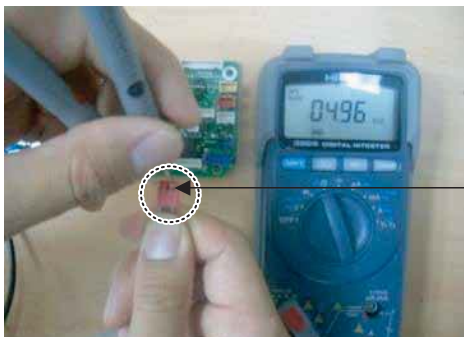
Measure the resistance of outlet pipe temperature sensor.
