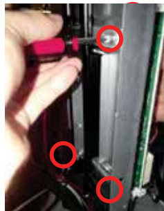
Figure 67: Detaching the Mounting Screws.
