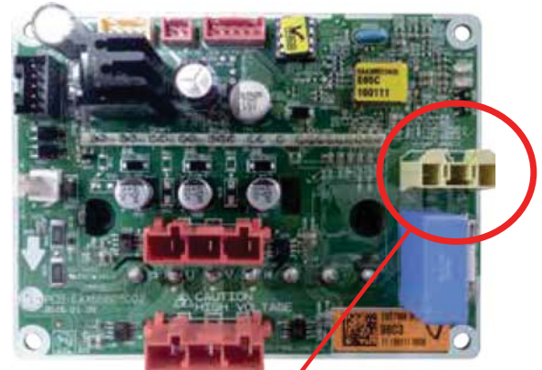
DC voltage connection.
