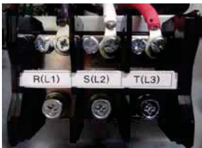
Measure input voltage.
