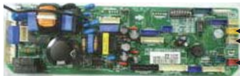
← CN-ROOM: Indoor Air Temperature Sensor ← CN-PIPE IN: Pipe Inlet Temperature Sensor ← CN-PIPE OUT: Pipe Outlet Temperature Sensor
