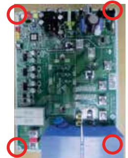
Figure 71: Removing the PCB.
