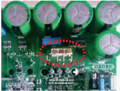
Figure 46: ARUN060GSS4 and ARUB060GSS4 Error No. 22 Compressor Terminal and Wiring Connections.
