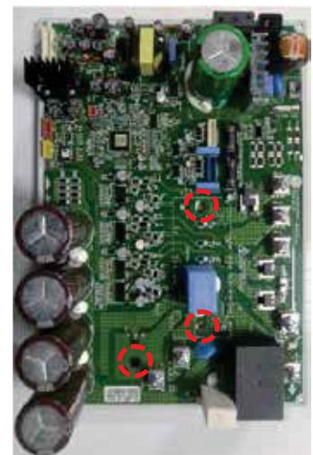
Figure 66: ARUN060GSS4 and ARUB060GSS4 Error No. 62 Checking the Connections (JIS Screwdriver Required).
