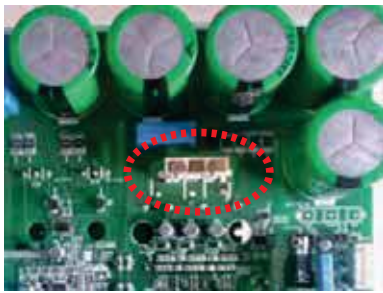
Figure 50: ARUN060GSS4 and ARUB060GSS4 Error No. 29 Compressor Terminal and Wiring Connections.
