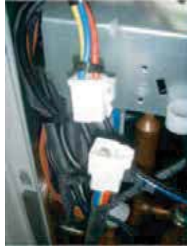
Figure 46: ARUN060GSS4 and ARUB060GSS4 Error No. 22 Compressor Terminal and Wiring Connections.
