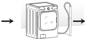
Connecting the drain line
