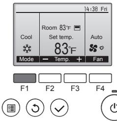
Press the [F1] button to go through the operation modes in the order of "Cool", "Dry", "Fan", "Auto", and "Heat". Select the desired operation mode.
