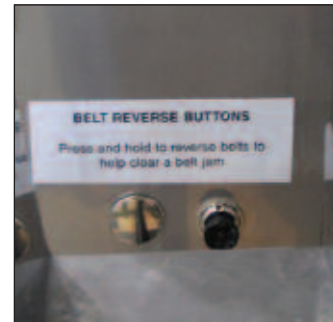
BEHIND CONTROL BOX Belt Reverse Button - Push to reverse the belt in case of a jam.
