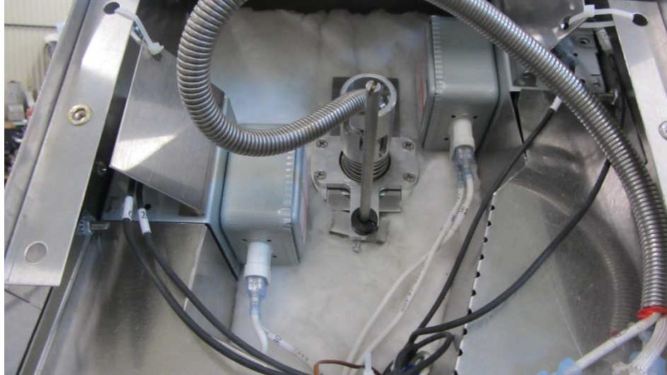
MAGNETRONS - MAGNETRON HIGH LIMIT SWITCHES - HEATER PLATE RELEASE MECHANISM & HEIGHT ADJUSTMENT COLLAR
