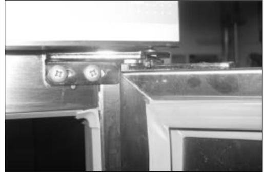
2. Remove screws for hinge.
