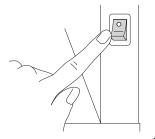
Unplug and let cool. Allow platen to cool for 60 minutes before cleaning. The plug removed from the outlet shall remain clearly visible to the operator during the maintenance procedure.
