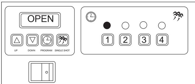
**OPEN** will be displayed when the thermocouple is "open" or not installed correctly. The unit will not call for heat.
