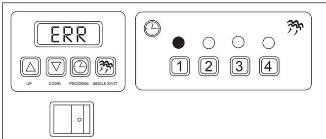
**ERR** will be displayed if there is a programming parameters error. If this message appears you will have to clear the current parameters. To clear the unit's current programming and reset the unit to its factory settings:
