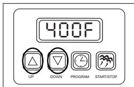
To verify or change the generator setpoint temperature, press and hold the **UP** and **DOWN ARROW** buttons simultaneously for three seconds. Then, raise or lower the temperature by depressing the **UP** or **DOWN ARROW** buttons. Release the buttons when the desired temperature is reached.
