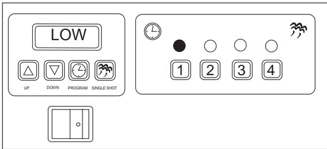
**LOW** will be displayed until the generator temperature exceeds 250°F (121°C).
