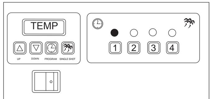
**TEMP** indicates the control cabinet temperature has exceeded 155°F (68°C) causing the unit to shut down.
