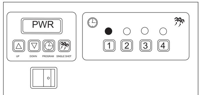
**PWR** will be displayed when the supply voltage is lower than 160 Volts AC or above 265 Volts AC.
