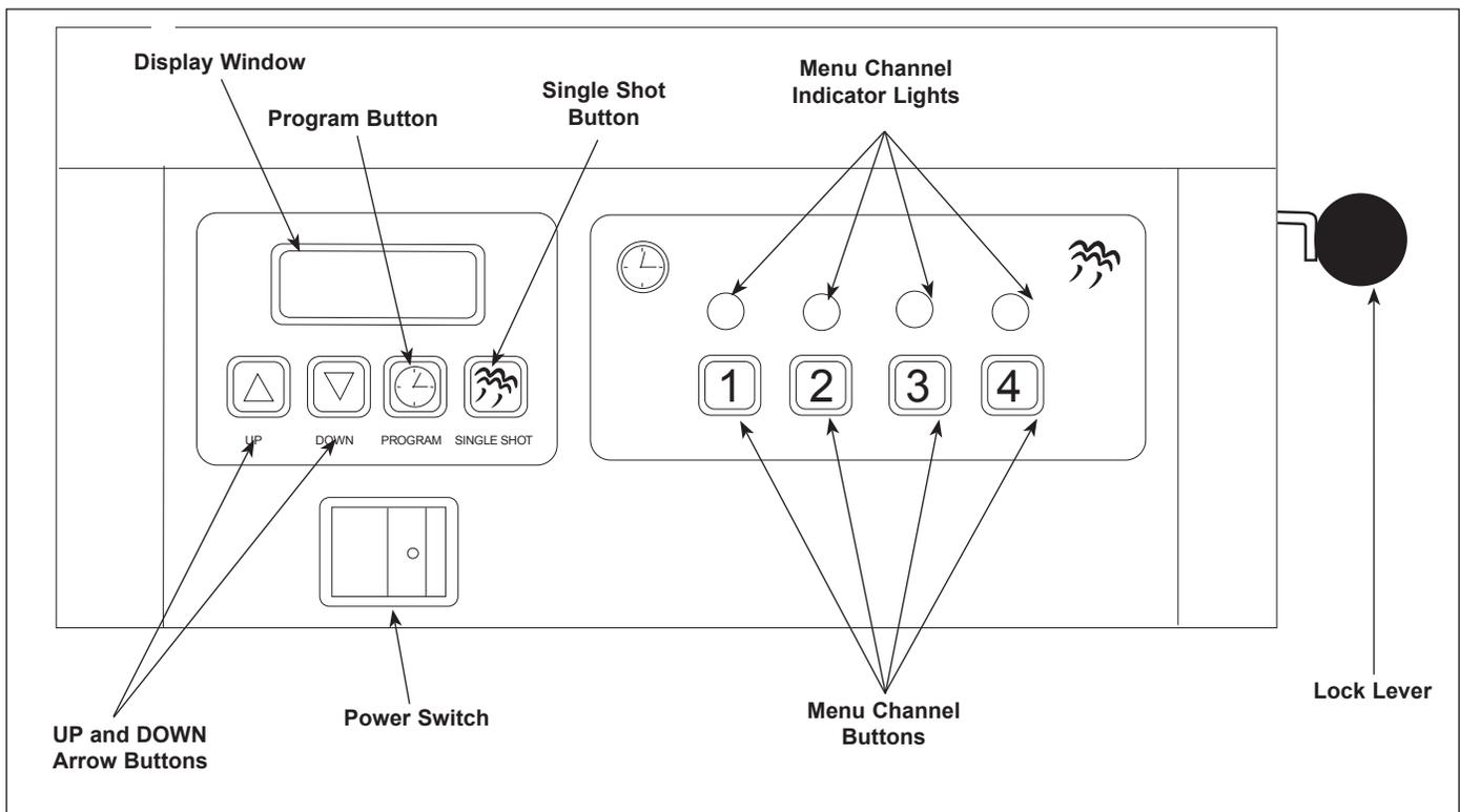
Figure 3. Operator Controls
