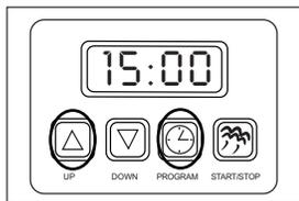
To Change the display from Fahrenheit (F) to Celsius (C), press and hold the **UP** arrow and the **PROGRAM** buttons simultaneously for three seconds. Repeat the process to reverse.
