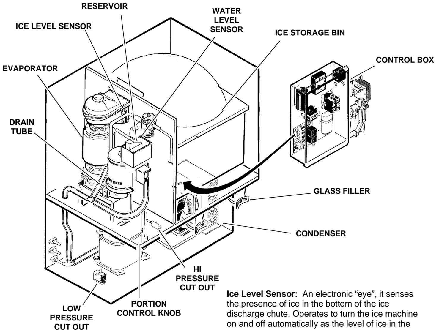
**Control Box:** Contains the electrical controls that operate the machine.
