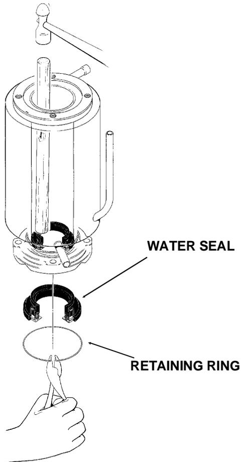
2. Replace the snap ring and pull the water seal down against it.
