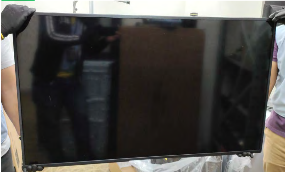
Always wear gloves during P-mod handling
