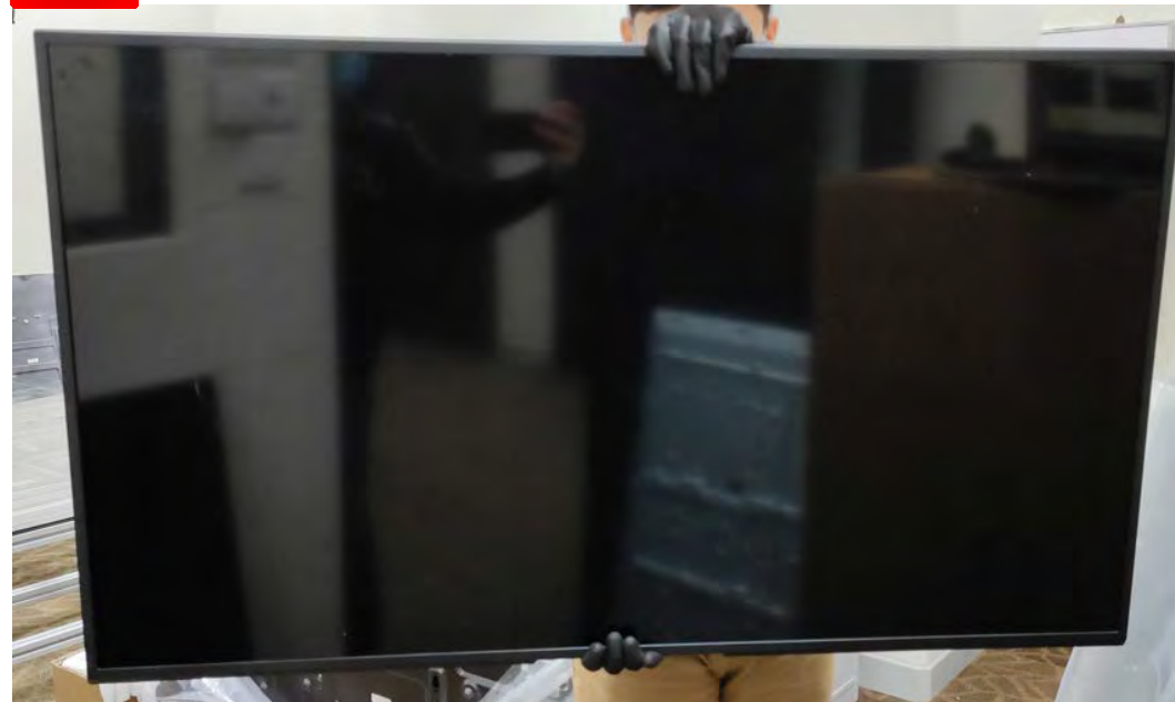
Carry P-mod at center area
