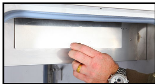
Convection blower wheel access for inspection/cleaning.
