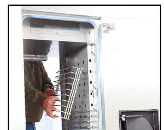
Removal of Rack Slides
