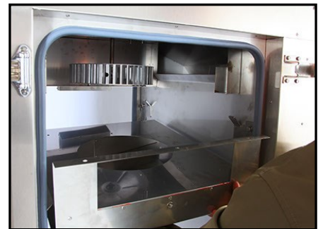
Removing shroud provides complete access to convection blower wheel for cleaning and/or removal of blower wheel.
