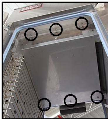
Six, 1/4-20 bolts secure blower wheel shroud into place. Remove these bolts to extract shroud from the top of the interior of the smoker.
