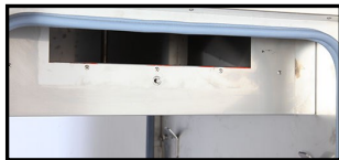
Convection blower wheel access for inspection/cleaning.
