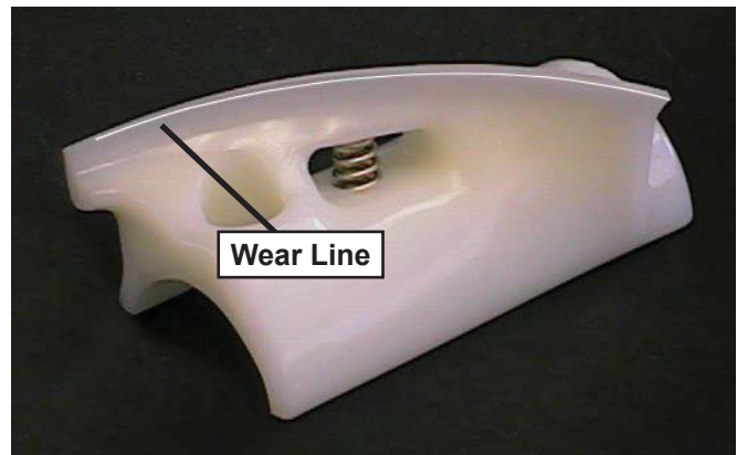
Figure 3-3 Auger Flight Wear
