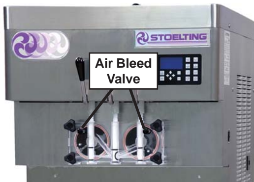
Figure 3-8 Air Bleed Valve
