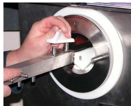
Figure 3-6 Installing Auger Blades
