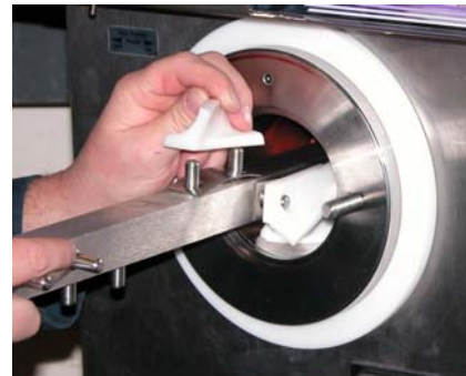
Figure 3-6 Installing Auger Blades
