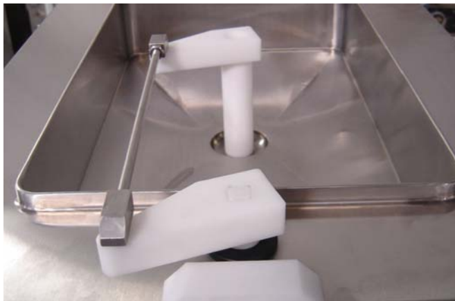
Figure 3-3 Flow Control Assembly
