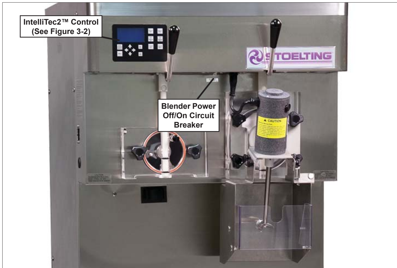
Figure 3-1 SU444 Freezer Controls
