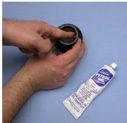
Figure 3-5 Lubricate Rear Seal
