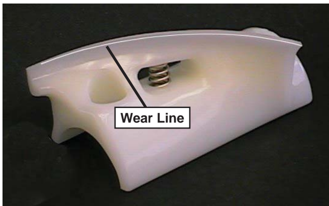
Figure 3-3 Auger Flight Wear
